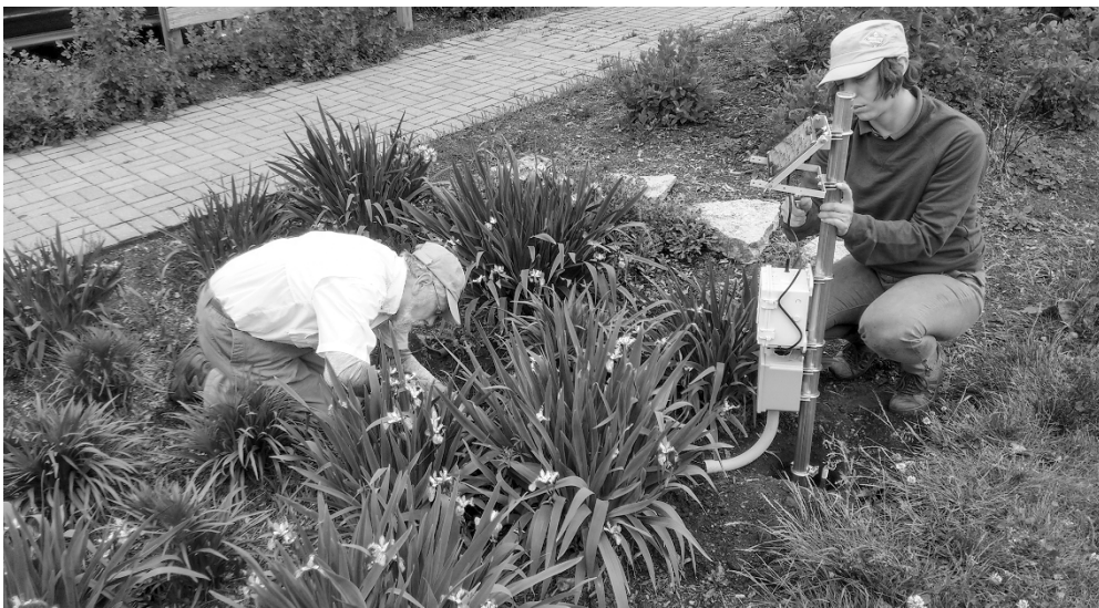
Figure 6-1. Vacant to Vibrant sites were outfitted with monitoring equipment to examine soil moisture fluctuations during natural storm events.
