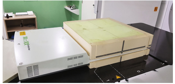
Fig. 2. (Color online) I'mRT MatriXX 2D ion chamber array with solid water phantom MULTICube.
