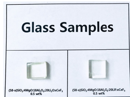
Fig. 1. (Color online) Glass samples : (58-x)SiO_2:4MgO:18Al_2O_3:20Li_2O:xCeF_3 (left) and (58-x)SiO_2:4MgO:18Al_2O_3:20LiF:xCeF_3 (right).
