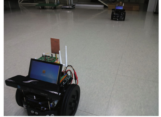
Fig. 5. (Color online) Two-wheeled mobile follower robot tracking a leader robot.
