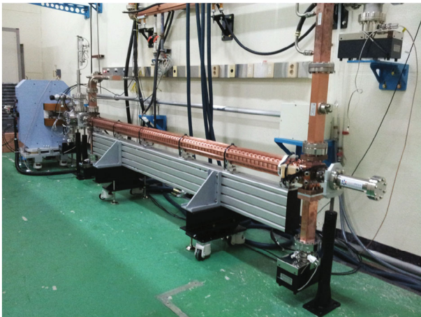
Fig. 8. (Color online) Photo of the tunnel of the high-power test facility for the accelerating structure (MHI structure).
