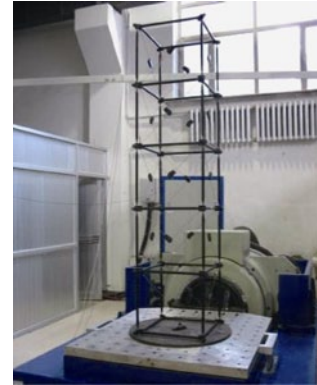
Fig. 22. Truss vibration experiment
