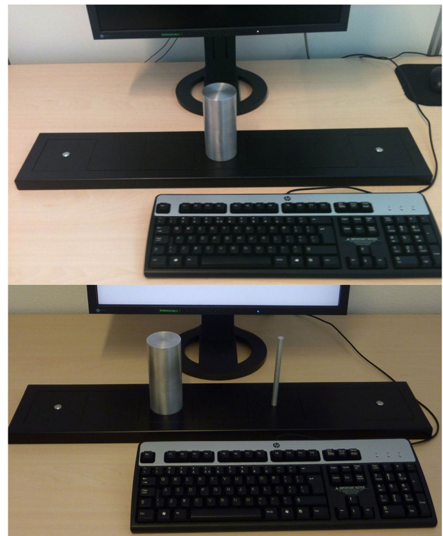
Fig. 2 The Grabbit setup for the go/no-go version (top) and two-choice version (bottom)
