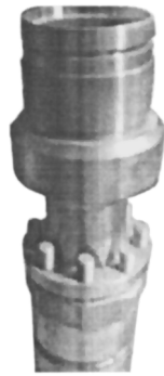
Fig. 2. Threaded joint for submersible centrifugal pumps, with pins.
