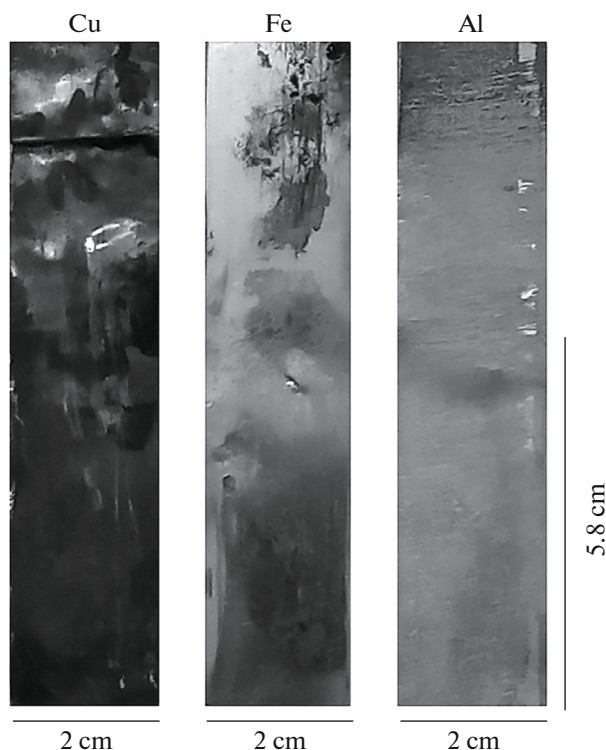
Fig. 1. Electrodes sheets with dimensions of the submerged surface area inside the dye solution in electrolytic cell.
