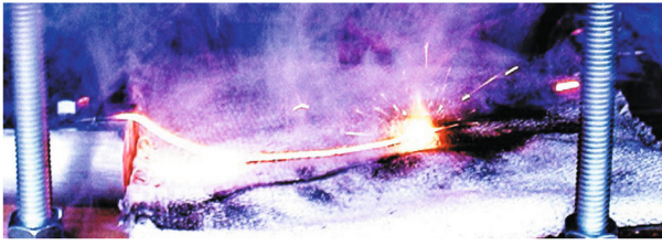
Fig. 1. Empirical demonstration of local melting of galvanized steel wire ( r_0 = 0.8 mm; l_0 = 320 mm; \Delta_0 = 5 \mu m) by discharge pulse of axial current i_0(t) of temporal form 9 ms/160 ms from powerful GIC ( \delta_{0m} \approx 0.37 kA/mm 2 ) in the zone of its only ( n = 1 ) hot longitudinal section \Delta z_{nh} \approx 7 mm long, which is cooling in air and on fire-resistant asbestos cloth.
