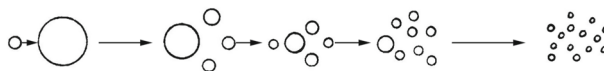
Fig. 3. Scheme of additional charging of slow big drops by small, fast, and strongly charged.
