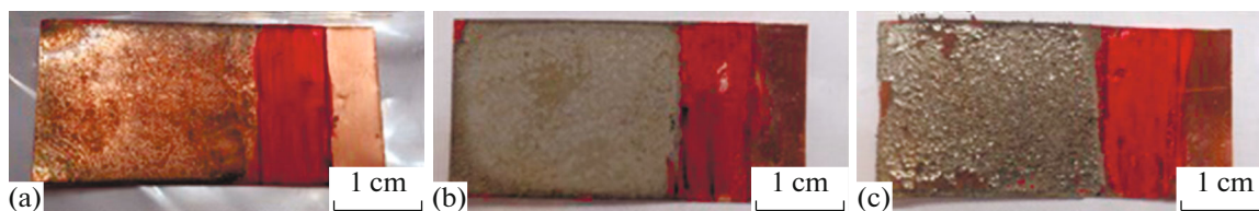
Fig. 17. Appearances of iron coatings deposited at different current densities and 60°C from bath with saccharin: (a) 1, (b) 5 and (c) 20 \text{A dm}^{-2} .
