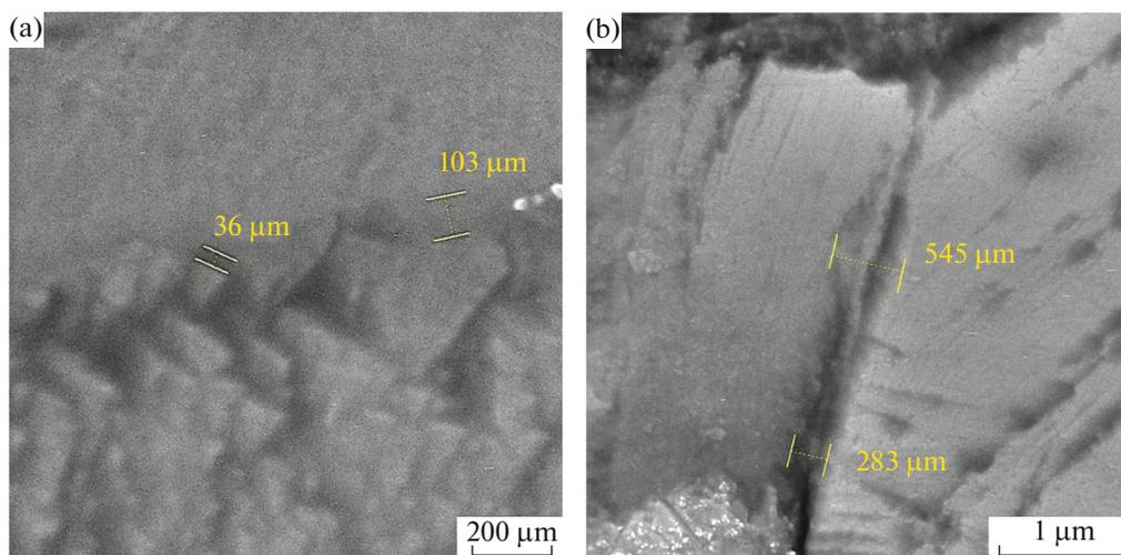
Fig. 2. Grain-boundary region in the structure of bronze BrO12 sintered at different holding times: (a) 60; (b) 120 min.
