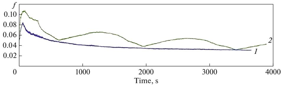
Fig. 4. Change in friction coefficient during friction of BrO12 bronze sintered for 5 min: (1) 4; (2) 20 MPa.
