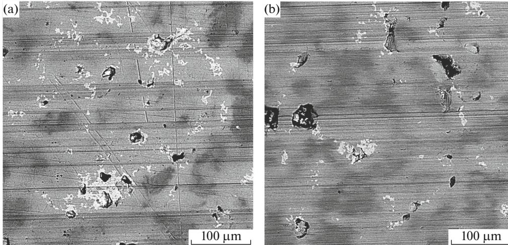
Fig. 5. Morphology of the friction surface of BrO12 sintered for 5 min (test time 4000 s): (a) 4; (b) 20 MPa.
