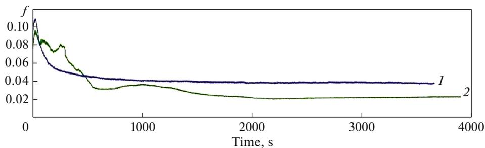
Fig. 6. Change in friction coefficient during friction of BrO12 bronze sintered for 60 min: (1) 4; (2) 20 MPa.
