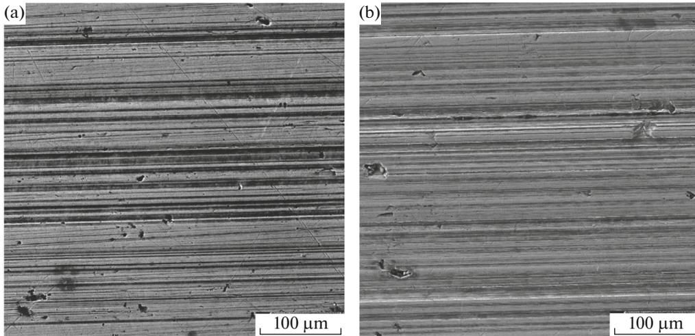
Fig. 7. Morphology of the friction surface of BrO12 sintered for 60 min (test time 4000 s): (a) 4; (b) 20 MPa.
