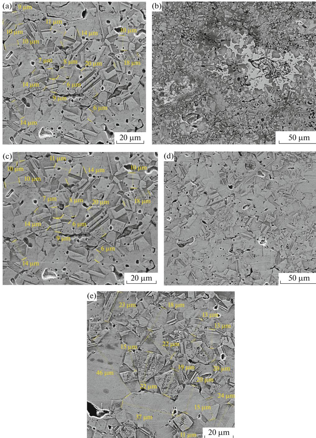
**Fig. 1.** Structure of BrO12 bronze sintered at different holding times: (a, b) 5; (c, d) 60; (e) 120 min; (a, c, e)  $\times 2000$ ; (b, d)  $\times 1000$ .
