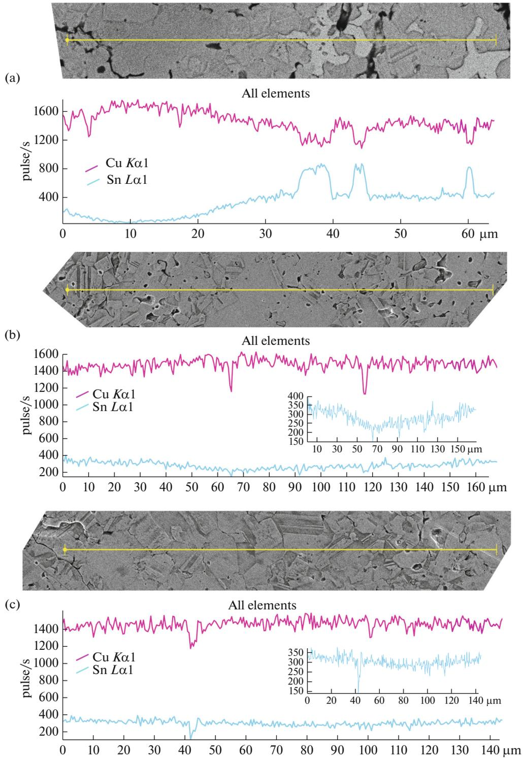
Fig. 3. Distribution of copper and tin in the structure of BrO12 bronze sintered at different holding times: (a) 5; (b) 60; (c) 120 min.
