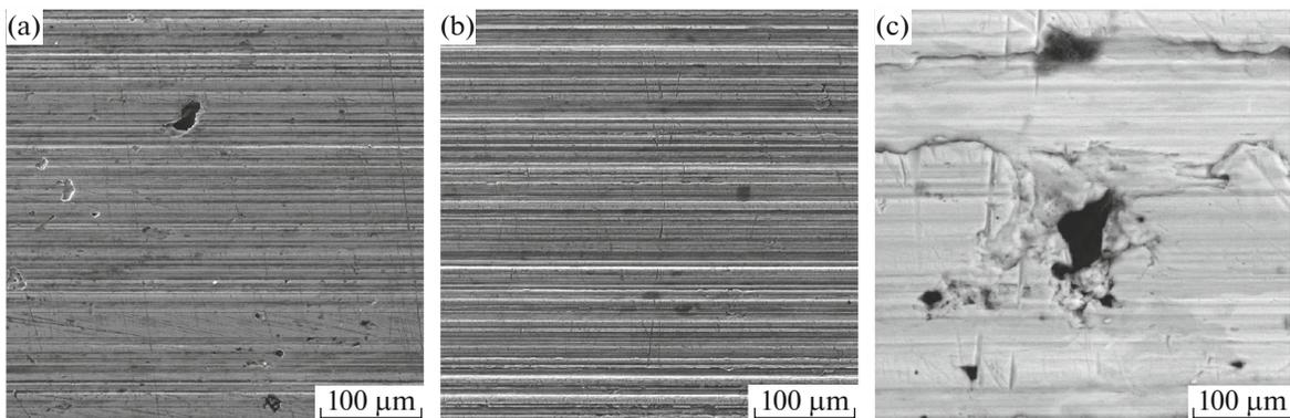
Fig. 9. Morphology of the friction surface of BrO12 bronze sintered for 120 min (test time 4000 s): (a) 4; (b, c) 20 MPa; (b) ×500; (c) ×5000.
