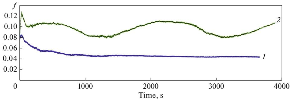
Fig. 8. Change in friction coefficient in time for BrO12 bronze sintered for 120 min: (1) 4; (2) 20 MPa.
