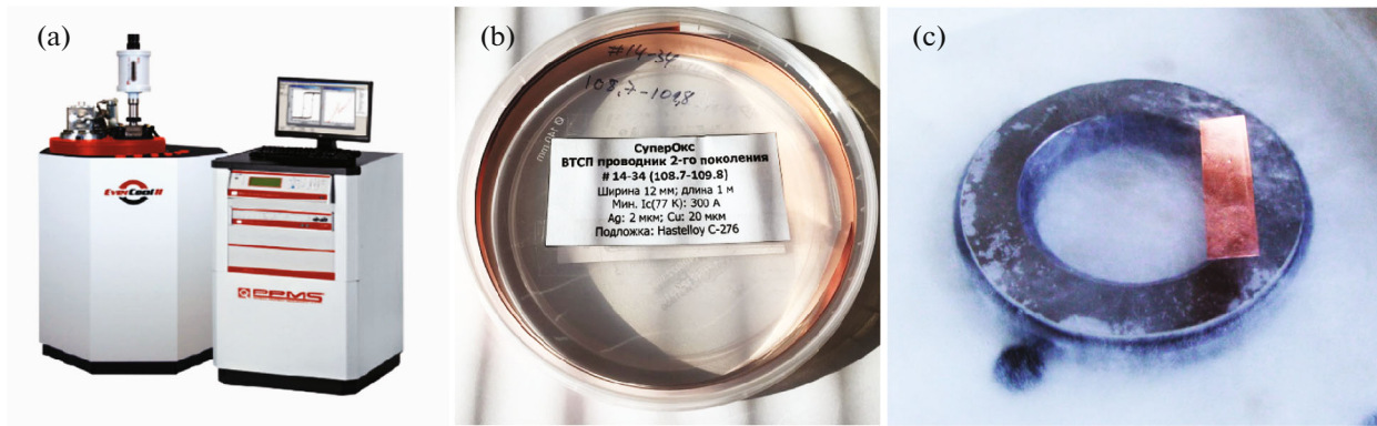
Fig. 1. (a) General view of the measuring complex PPMS-9 (Quantum Design), (b) HTSC tape manufactured by SuperOx, and (c) levitation of a HTSC tape in a magnetic field at T \sim 80 K.
