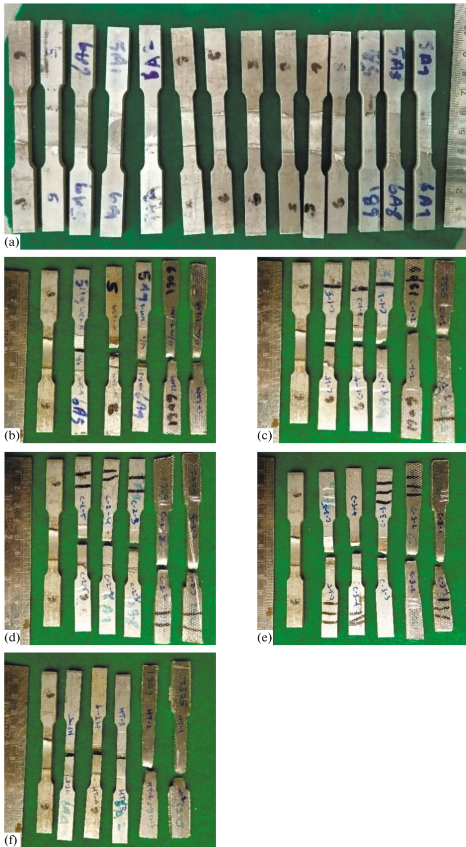
Fig. 8. (a) Tensile specimens; (b) AW specimens; (c) C-1 specimens; (d); (e) C-3 specimens; (f) HT specimens.
