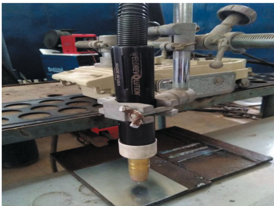
Fig. 1. Image of SpinArc GMAW torch used for this work.
