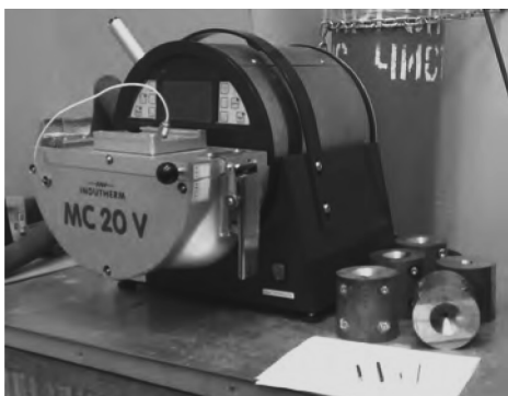
Fig. 1. Installation for gravitational casting of the melt heated with the help of an inductor into copper molds in vacuum or argon. Photograph is presented by authority of the Department of Materials Science of Nonferrous Metals at the National University of Science and Technology MISiS. Molds and BMG castings are seen on a table.
