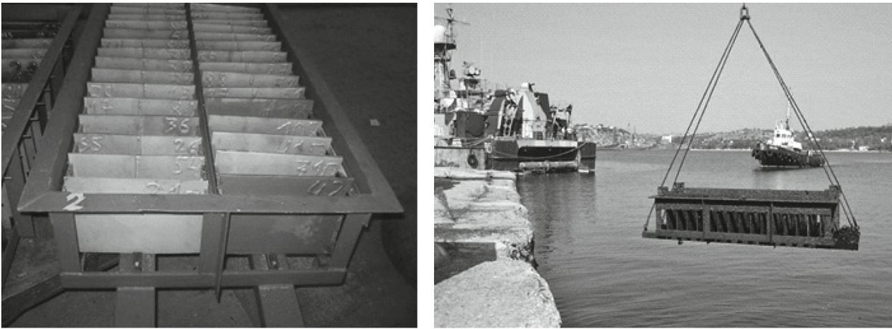
Fig. 3. Field tests for immersing samples in seawater with the use of a cassette.
