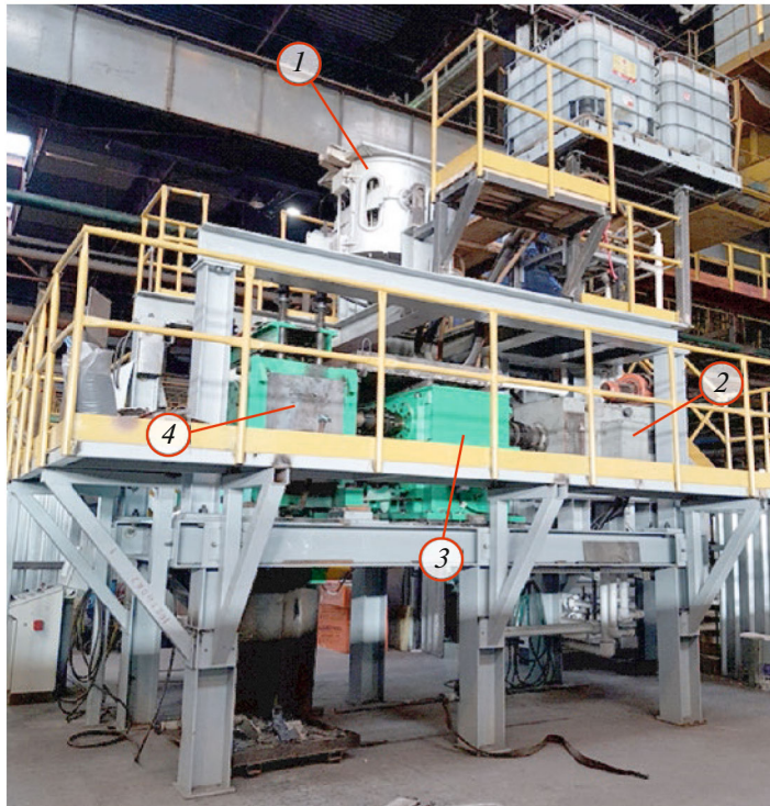
Fig. 5. Continuous casting and deformation section: (1) induction furnace; (2) DC motor; (3) synchronizer gearbox; (4) unit frame.
