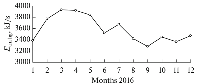
Fig. 5. Change in the total mechanical energy of the hearth gas flow at the 5000-m 3 furnace by months in 2016.
