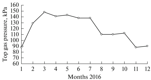
Fig. 1. Change in excess pressure of the top gas at the 5000-m 3 furnace by months in 2016.
