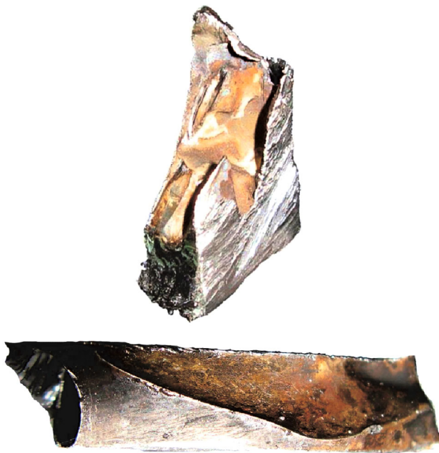
Fig. 5. Samples cut at the defect site, transverse (top) and parallel (bottom) to the rolling direction of the steel sheet.
