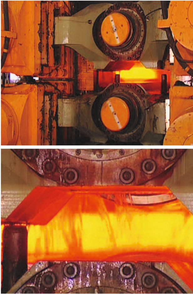
Fig. 1. Hot steel strip between rollers in a mill.
