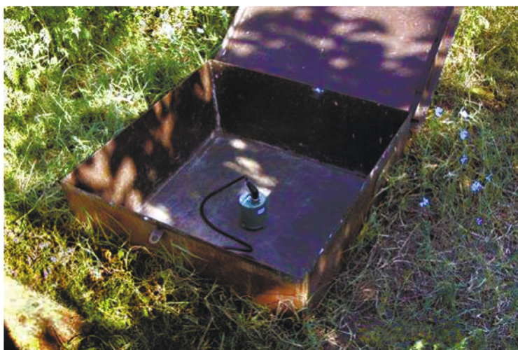
Fig. 2. General view of bunker with Trilium TC120-SV1 seismometer in standard housing. Eremizino-Borisovskaya Station.
