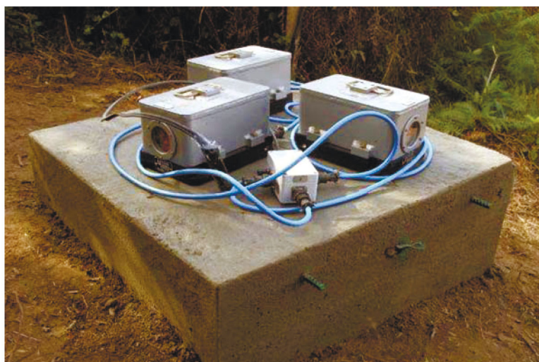
Fig. 3. Set of SM-3KV short-period seismometers on pedestal in metal cover. Veseloe station.
