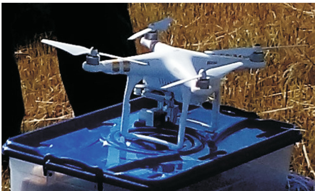
Fig. 2. DJI PHANTOM 3 PROFESSIONAL drone used for aerial photography.
