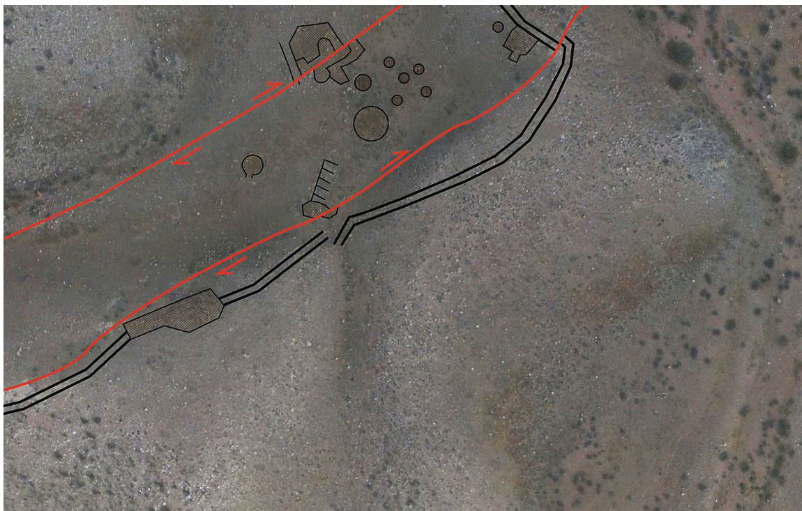
Fig. 15. Parallel faults in temple part of complex with destruction of building foundations, top view.
