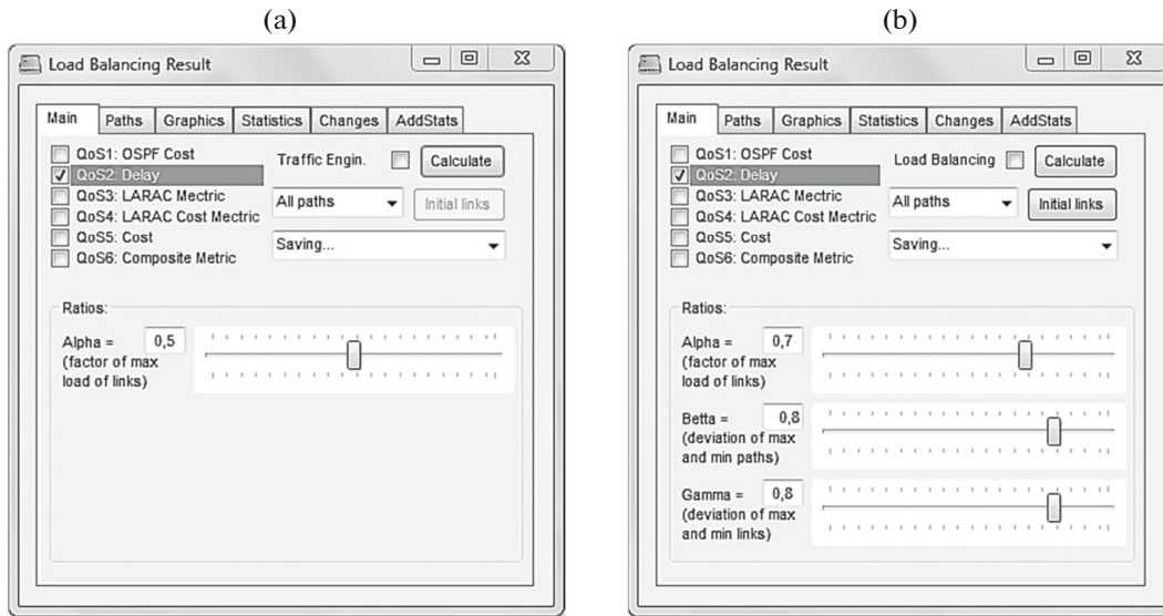
Fig. 10. Dynamic load balancing windows: (a) Window of Alpha coefficient control for YATE-module; (b) Window of Alpha, Beta, Gamma coefficients control for EDLBA.
