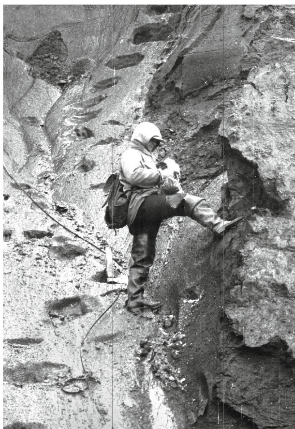
Fig. 2. Sampling for isotope-geochemical analyses from the Late Pleistocene syngenetic ice wedge of Ayon yedoma. Photo by Yu.K. Vasil'chuk.
