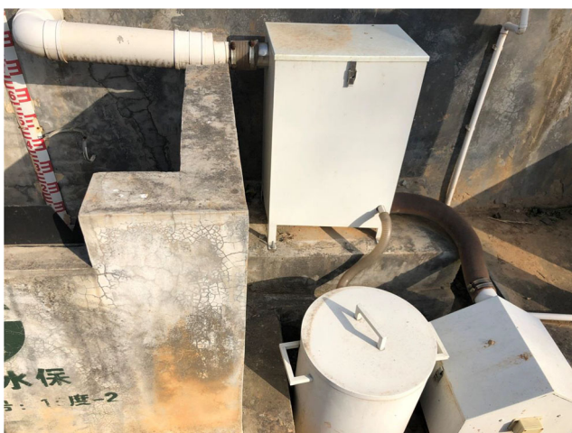
Fig. 2 Schematic diagram of runoff automatic monitor
