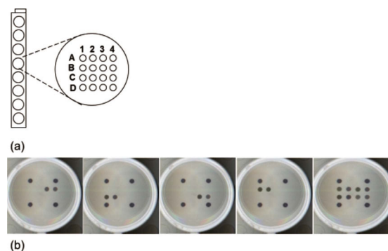
Fig. 2 (a) Pattern of immobilized probes. A1, A4, D1, D4, Hybridization positive control; B1, B2, E. coli O157:H7; B3, B4, Salmonella ; C1, C2, Shigella ; C3, C4, L. monocytogenes . (b) Specificity of the micro-plate chip assay for four pathogens. PCR amplicons from one of four pathogens were hybridized with chip. From left to right: Salmonella , Shigella , L. monocytogenes , E. coli O157:H7 and simultaneous detection of four pathogens, respectively.
