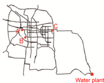
Fig. 1 Locations of sampling sites (locations A, B, and C were chosen by considering their similarity in terms of water quality, flow velocity, water age, and pipe age)
