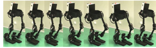
Fig. 15 Snapshots of a self-balanced walking experiment on a flat terrain
