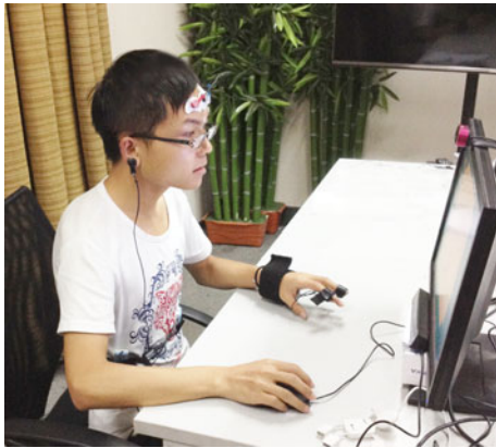
Fig. 2 Multimodal sensors placed on the volunteer in the experiment
