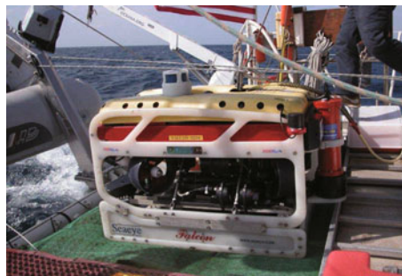
Fig. 1 Remotely operated vehicle used for image acquisition: Seaeye Falcon
