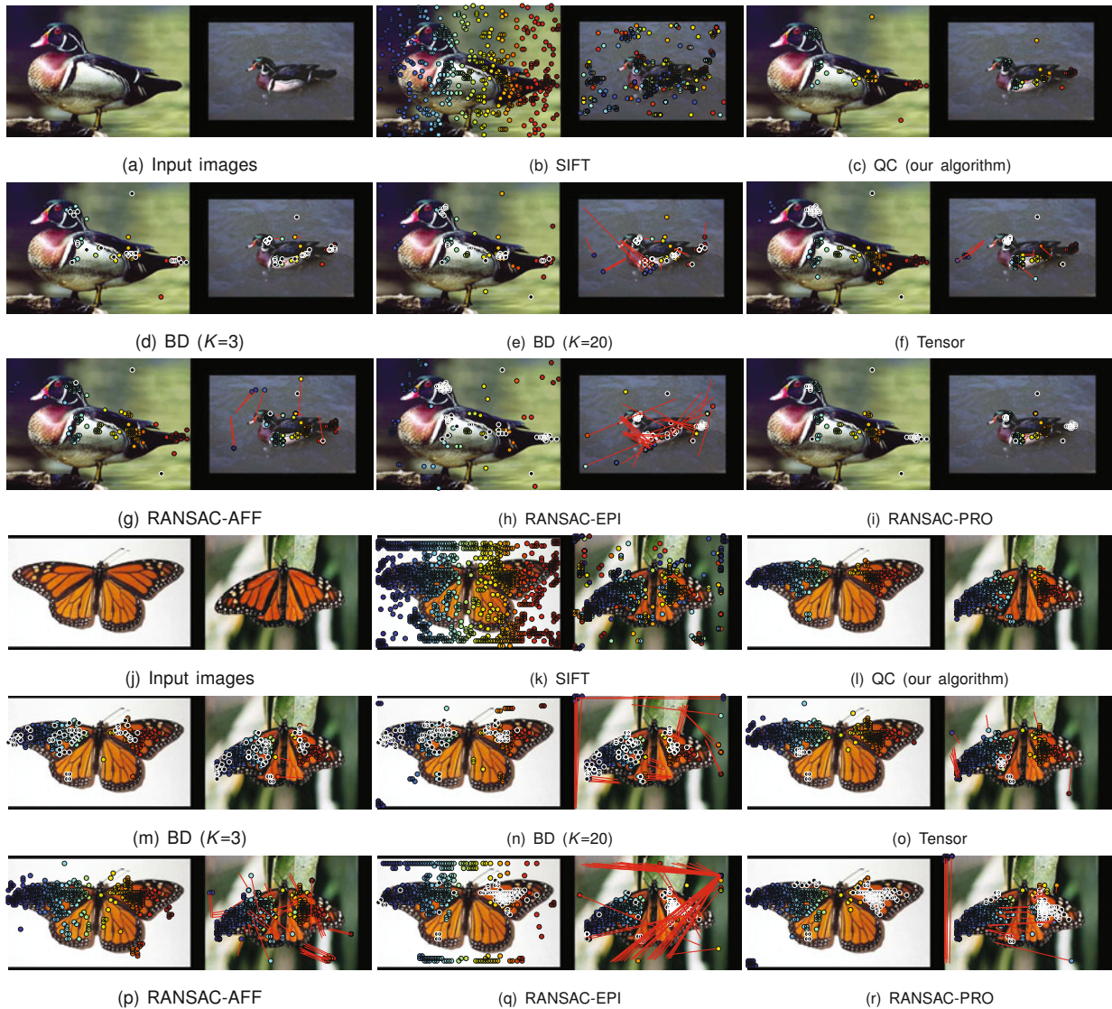
Fig. 5 Experiments on real images of different animals of the same species: red lines show the errors between selected correspondences and ground-truth correspondences and the black disks in the results are used to visualize the pairs selected by our method but missed by other methods (see caption in Fig. 3 for details). The images were taken with permission from Lazebnik et al. (2004; 2005) (References to color refer to the online version of this figure)
