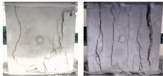
a) Teflon friction reduction b) Wax paper friction reduction
