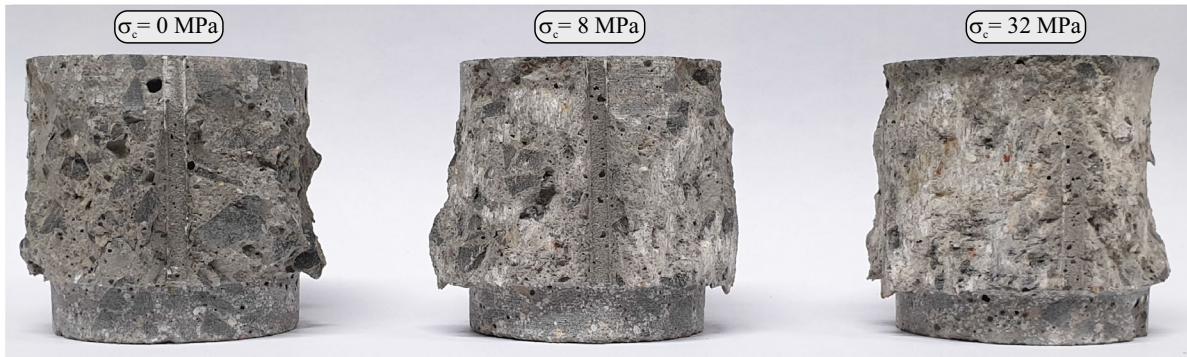
Fig. 6 Inner concrete cylinders after monotonic testing with different lateral compressive load levels
