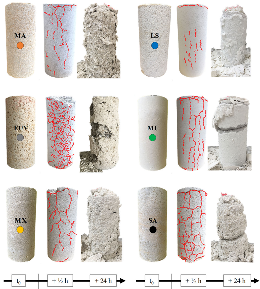
Fig. 12 Effect of the 800 °C heating–cooling cycle on limestone specimens ( \Phi 4 \times 8 cm): at initial state ( t_0 ); 30 min after being removed from the furnace (+ ½ h); after 24-h exposure in a monitored room at 50% and 20 °C (24 h). Red lines correspond to macroscopic cracks
