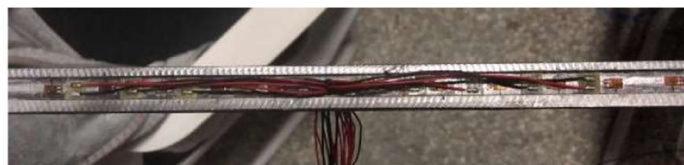
Fig. 6 Distribution of steel strain gauges: a size of the gauge distribution region and b photo of the attached gauges (unit: mm)
