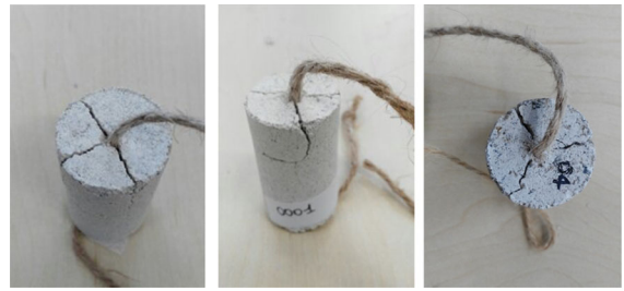
Fig. 6 Evidence of longitudinal cracks; samples tested for the interface failure mode
