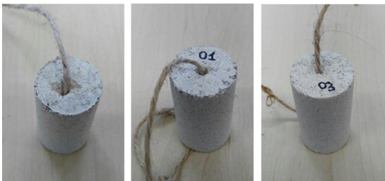
Fig. 5 Evidence of groove around the fibre; samples tested for the matrix failure mode
