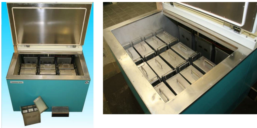
Fig. 3 Reactor generating 60 °C and 100% humidity
