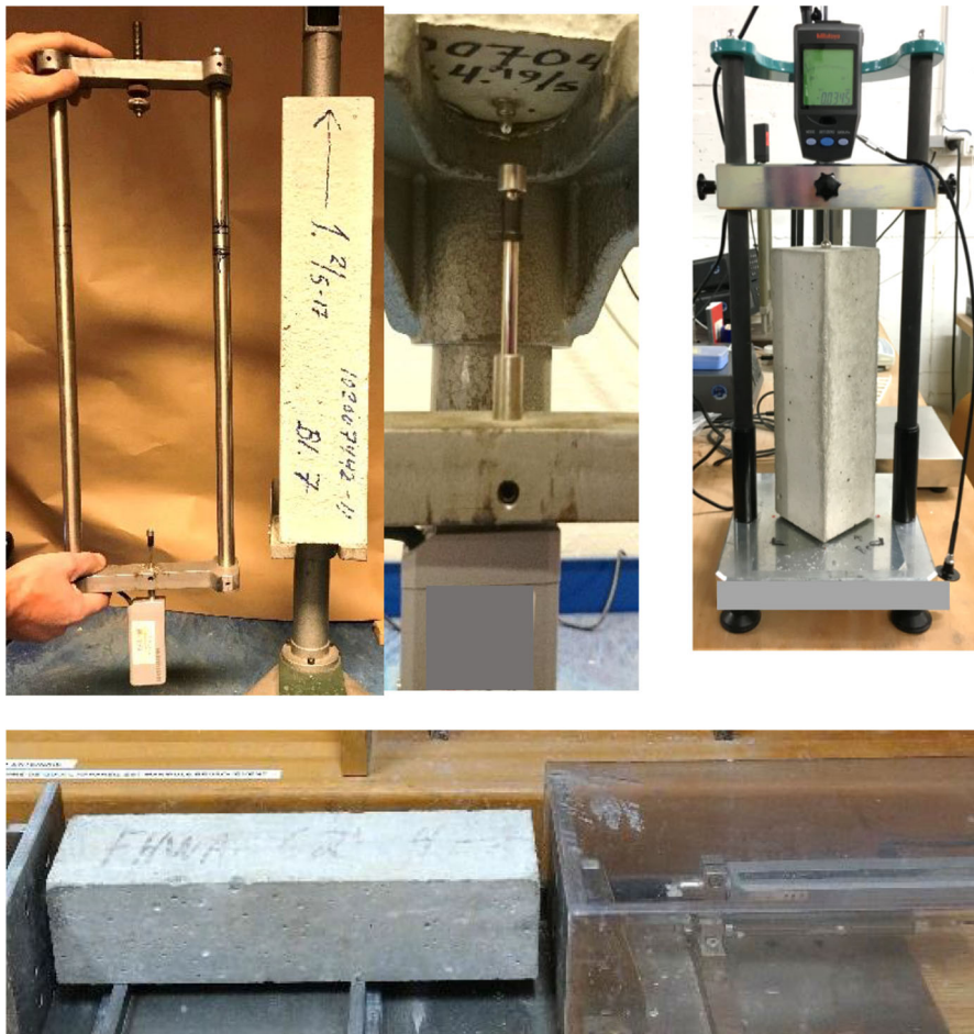
Fig. 1 Example of length comparator with gauge mounted rigidly in a vertical orientation (above) and horizontally (below)
