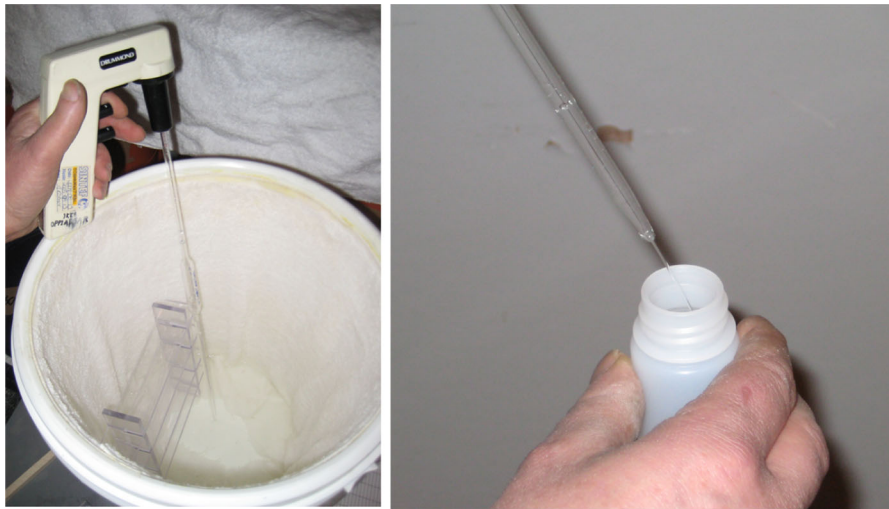
Fig. 8 Sampling of water in a container by use of a pipette (left). Plastic bottle for storage of the water sample (right)
