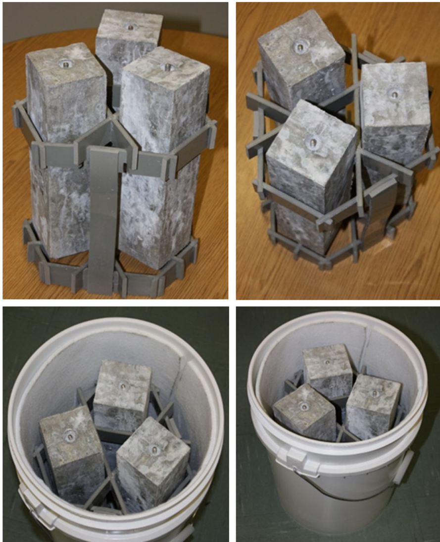
Fig. 5 Concrete prism specimens in the storage container. A plastic rack is used to hold the prisms in a vertical position in the plastic pails
