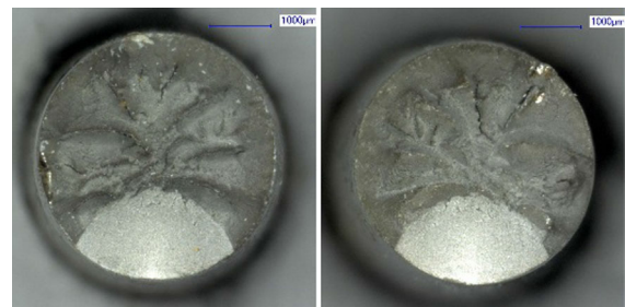
Fig. 16 Fractured wire surface of specimen mDSV-B-500-1
