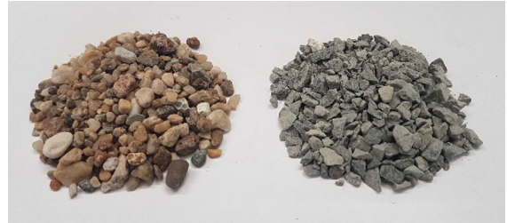
Fig. 9 Different coarse aggregate: Gravel (left) and basalt grit (right)
