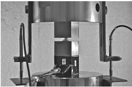
Fig. 4 Instrumented aluminum cube, with the i-BSJ, between the machine steel platens
