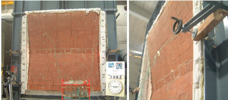
Fig. 6 Deflected shape of a masonry wall at the end of the fire test
