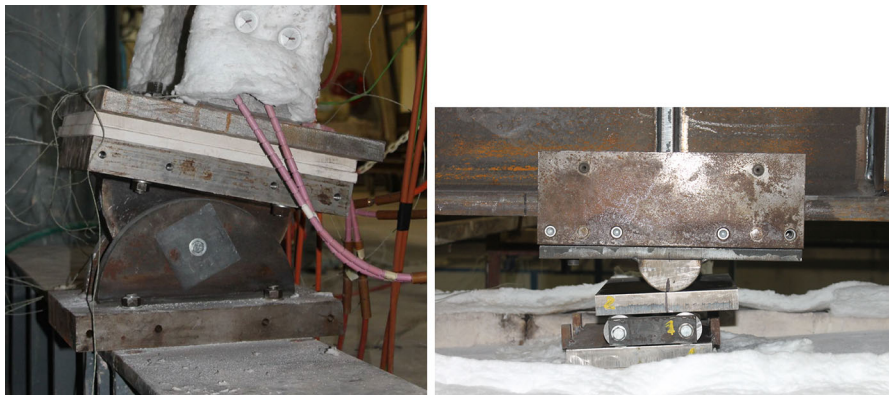
Fig. 1 Hinge connection used for a column test (left) and rolling hinge support used for a beam test (right)
