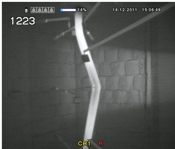
Fig. 4 Deflected shape at the end of a fire test after exceedance of the deflection criterion
