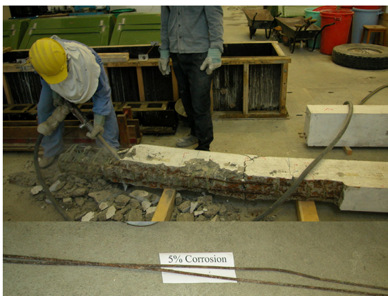
Fig. 4 Extracting the corroded bars after the test for evaluation of the actual mass loss
