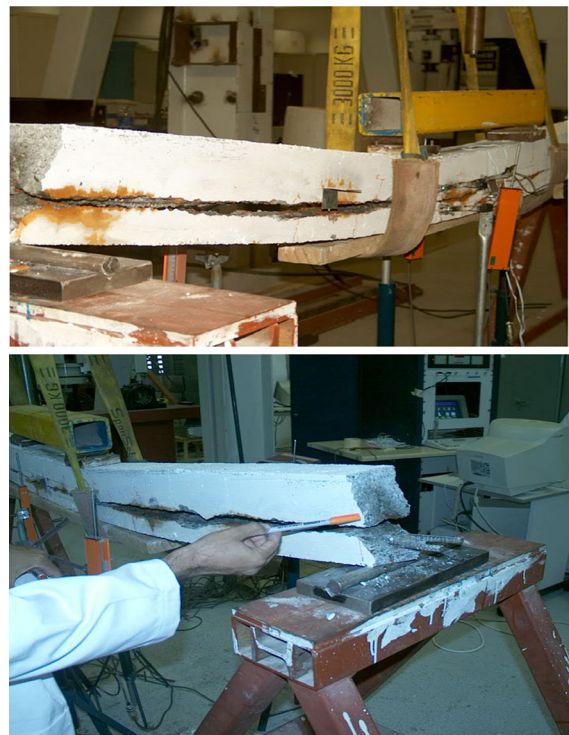
Fig. 6 Bond failure of beam AC5&AC7.5
