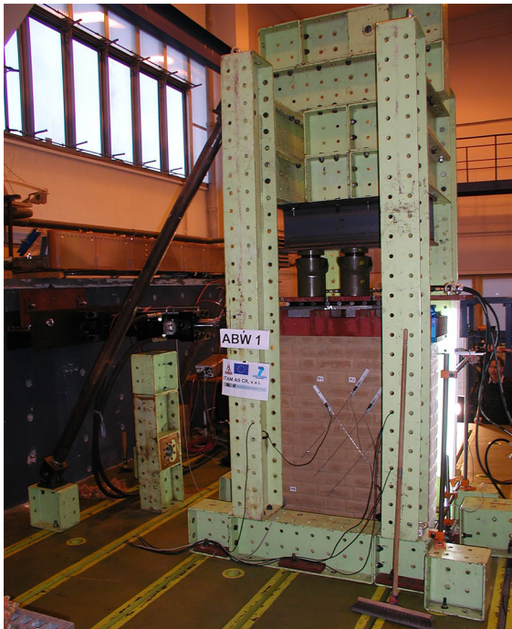
Fig. 3 Testing rig with the specimen
