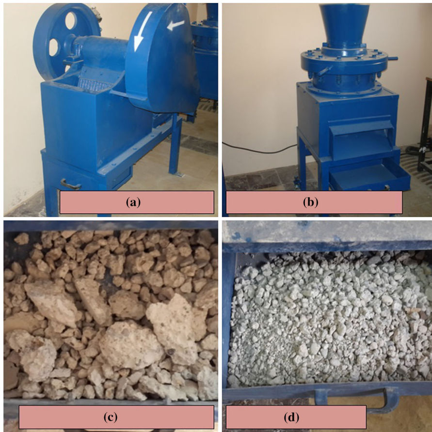
Fig. 1 Two-stage crushing system: a primary crusher ( jaw ), b secondary crusher ( cone ), c feliceous shaped aggregate, and d recycled aggregate
