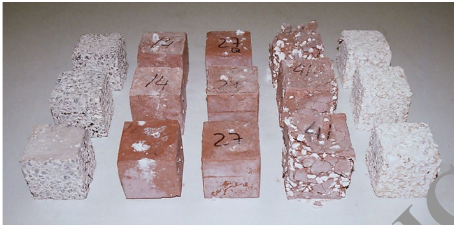
Fig. 6 Sulphuric acid attack. Specimens before detachable particles have been removed
