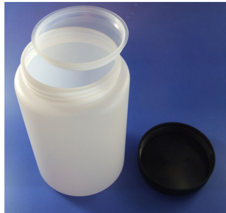
Fig. 1 Example of double-closure container, with \Phi 10\text{cm} \times 15 cm high
