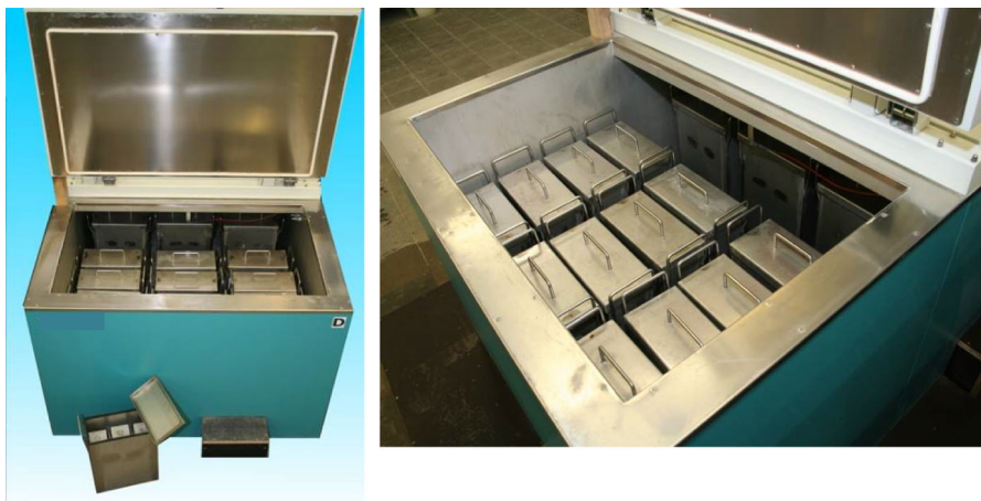
Fig. 3 Reactor generating 60 °C and 100% humidity
