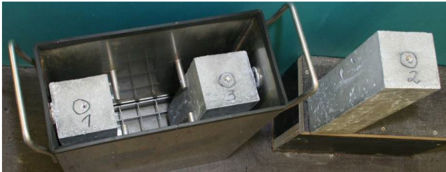
Fig. 4 Sealable containers suitable for the AAR-11 for storing concrete prisms (dimensions in mm)
