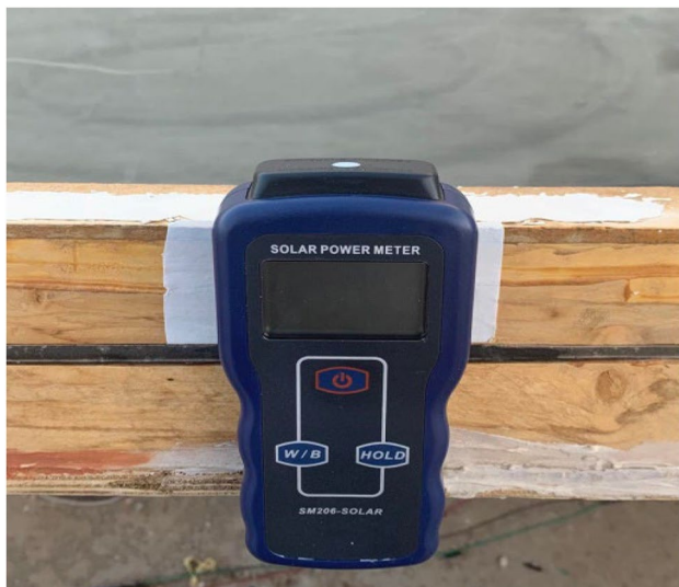
Figure 6. Solar irradiance meter utilized during the experimental work.
