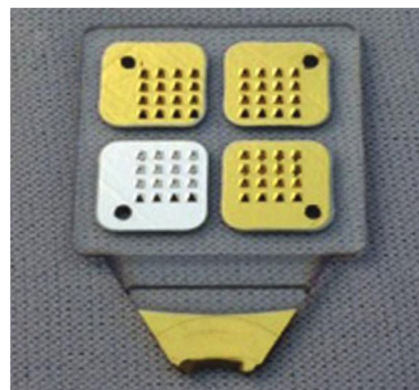
Figure 8. Polycarbonate structure of four 4 \times 4 microneedle arrays metallized with gold and silver. Reprinted from Ref. 85, distributed under the terms of the Creative Commons CC BY license.
